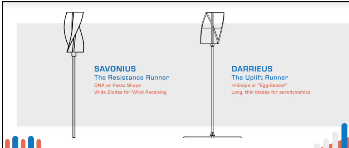
Fig7.11: Anatomy and Operation of a Vertical Axis Wind Turbine
