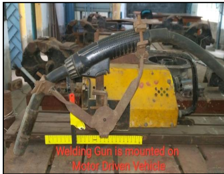
Fig. 9.2: Welding Gun mounted on Motor driven vehicle
